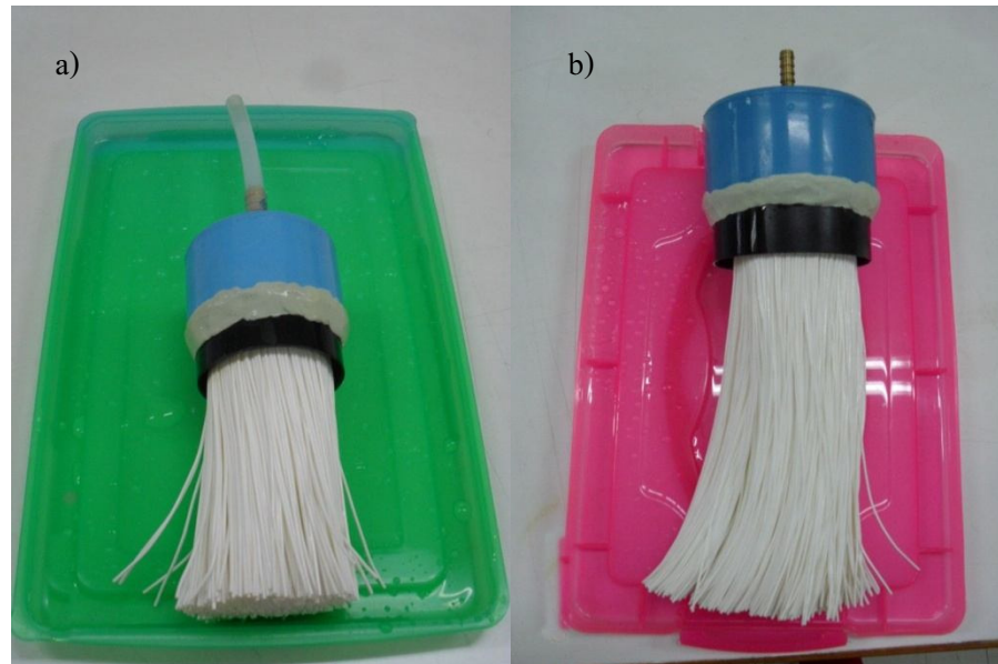
Figure 3.5 Hollow fiber membrane modules a) ultrafiltration membrane (UF) and b) microfiltration membrane (MF)
