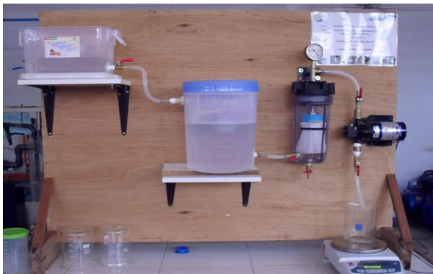
Figure 3.8 The pictorial of experimental set-up of ultrafiltration process
