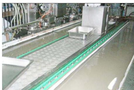
Moisture in the atmosphere contaminated into the open system
