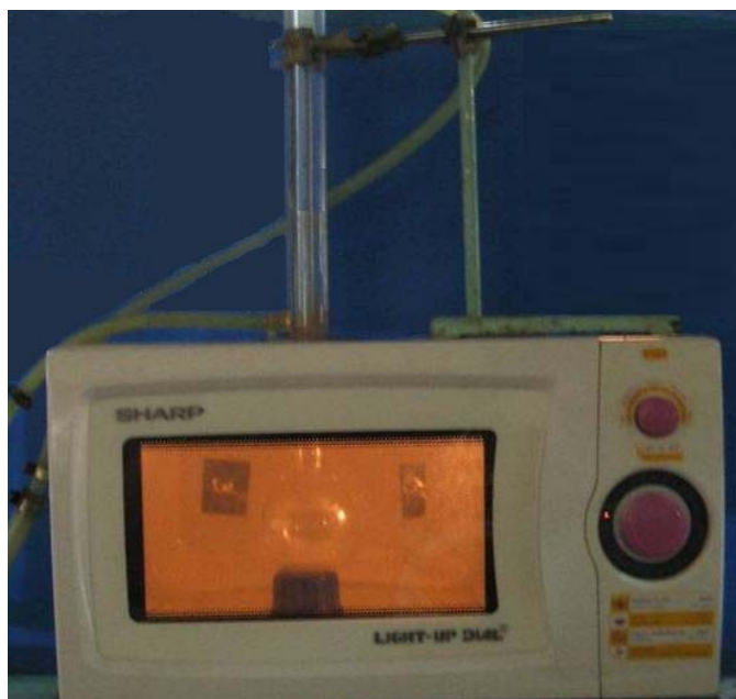
Figure 3.2 The microwave system for ethyl ester production
