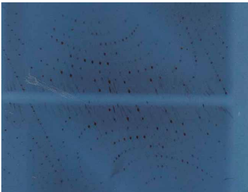
Figure 30 The zero layer Weissenberg photograph of [Cu 4 (ptu) 6 I 4 ] 2 .
