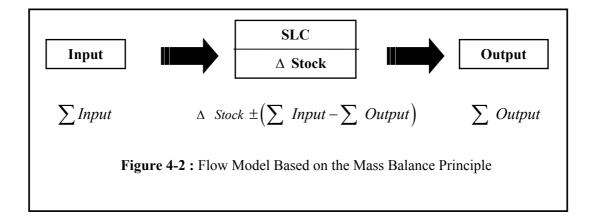
Figure 4-2 shows the principle of the mass balance, which is based on the input, stock, and output of the system. Substance quantities can change over time but the objective of the system is to maintain the balance between input and output. The input of substance should not exceed the output and dispersion into the environment should be avoided by keeping the substance stored in the economic system.
